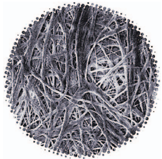
The microfiber technology of DuPont™ Tyvek® used for graphics applications offers high-strength, durability and opacity resulting in the best characteristics of paper, film and fabric in one substrate. (Shown 200 times.)
